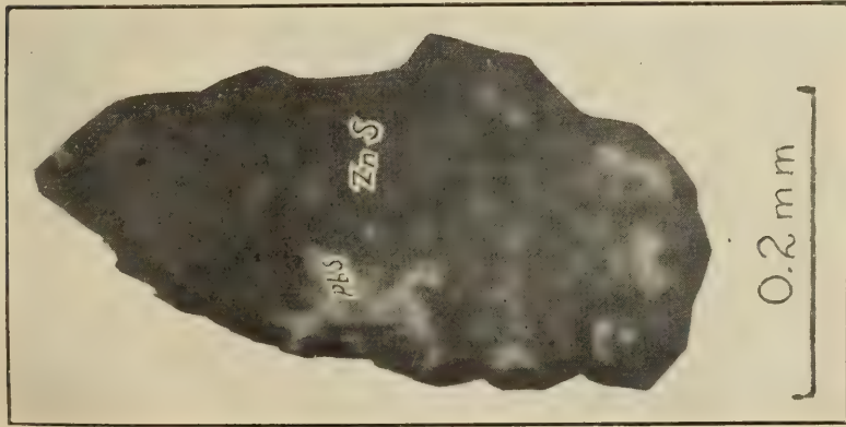
4. A GRAIN OF ORE 1, SHOWING INCLUSIONS OF GALENA IN SPHALERITE.
